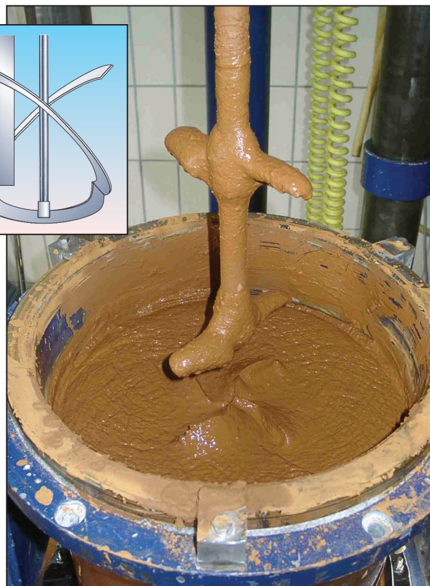
FIGURE 6. Pilot plant testing of high-viscosity slurries, such as this mineral-ore slurry with a yield stress, is highly recommended for good mixer-design performance
